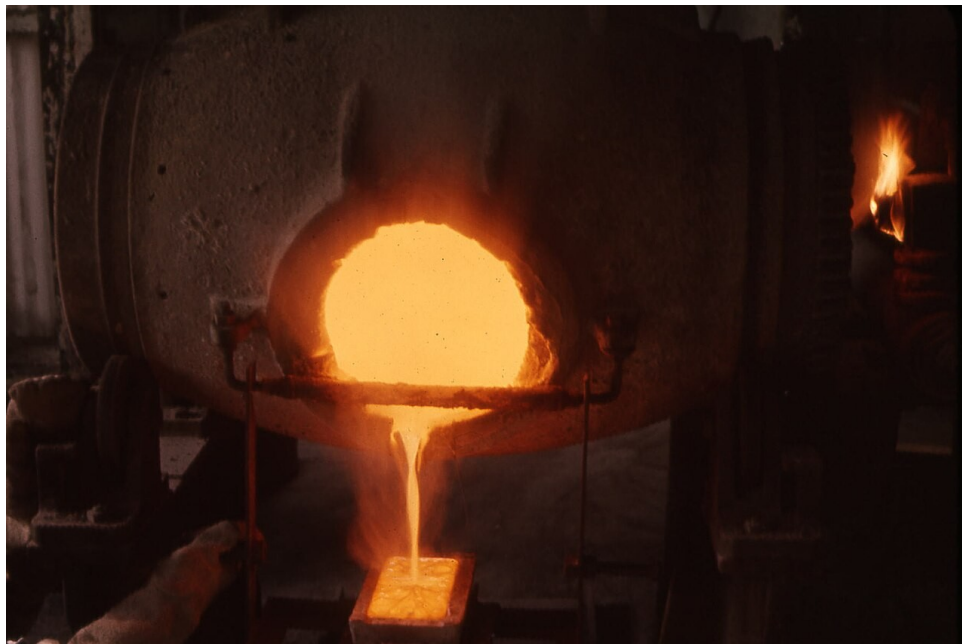
Figure 8 - Pouring molten gold into ingot mold at the former La Luz Mine
