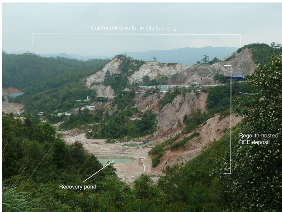
Figure 4 – Regolith Hosted REE Deposit , China Credit: Kevnmh, Creative Commons Attribution-Share Alike 4.0 International license
