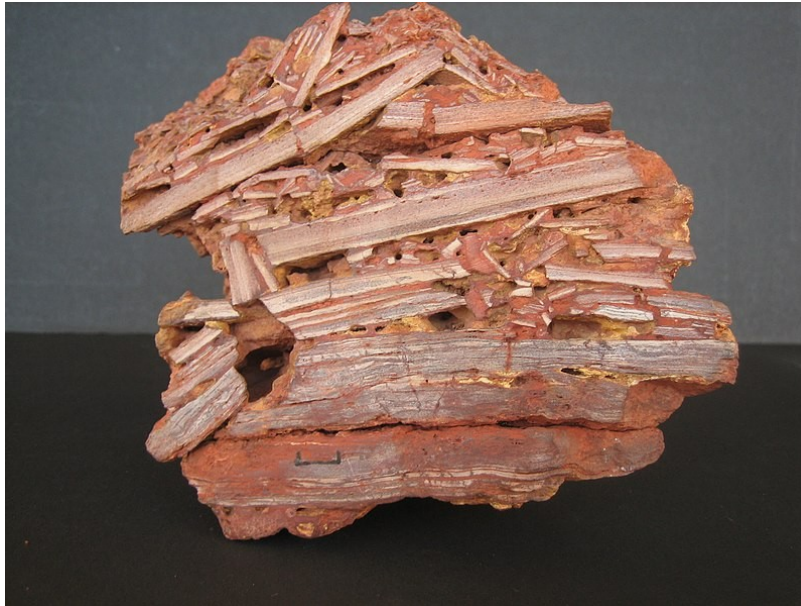
Figure 7 – Bauxite Specimen with Relict Stratification of the Parent Rock (slate), Fria, Guinea Credit: Creative Commons Attribution-Share Alike 3.0 Unported license
