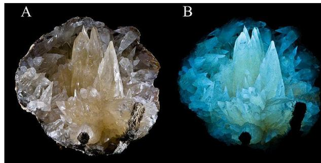
**Figure 1 - Calcite Under Regular & UV Light**
